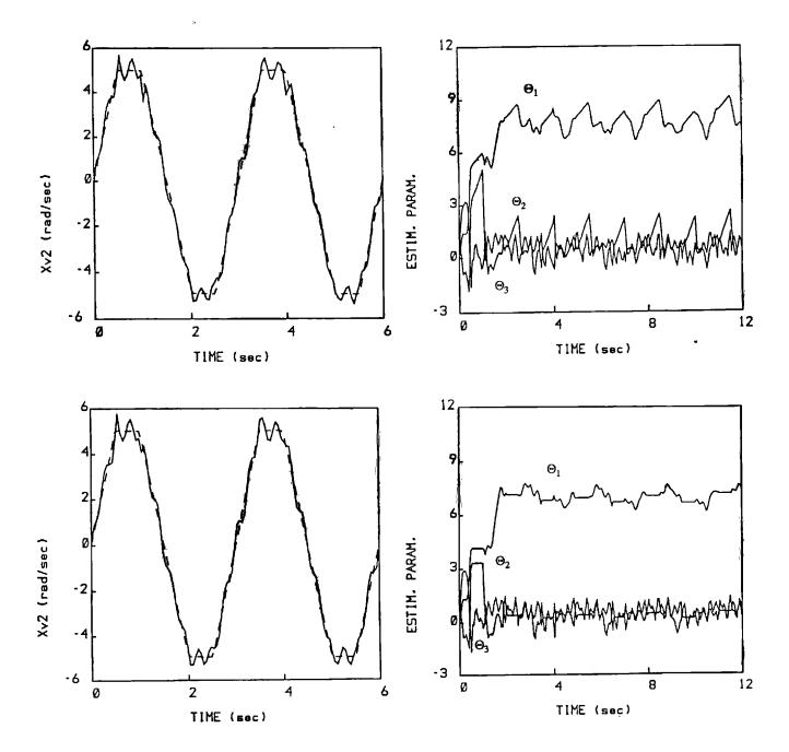
Simulation results revealed that the position and velocity response of the second axis contained a larger tracking error than those of the first axis. This is expected, since the same desired position and velocity trajectories were chosen for both axes, and the second axis has a smaller inertia than the first one. Hence the
